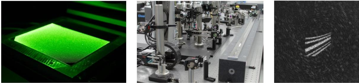
*Insights from the laser laboratory at Fraunhofer ISE: laser structuring (left) and optical setup for recording the ablation process at high temporal resolution (center) and flexible beam shaping using phase modulation (right).*
