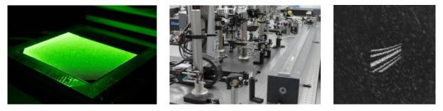
Insights from the laser laboratory at Fraunhofer ISE: laser structuring (left) and optical setup for recording the ablation process at high temporal resolution (center) and flexible beam shaping using phase modulation (right).
